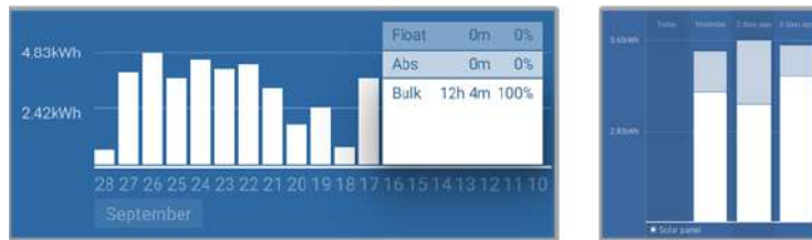
Left: Example of a system that is spending all its time in the bulk stage. Right: Breakdown of the charge stages - The system spends time in bulk and in the absorption stage.
