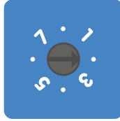
Rotary switch set to position 2
