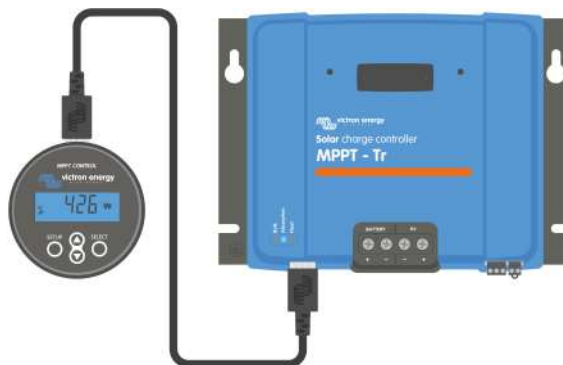
Connect the display to the solar charger via a VE.Direct cable
