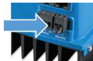
Remote connector with the wire loop.
