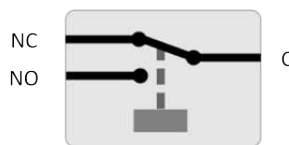
Relay configuration (not energised).
